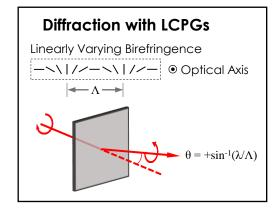
Meadowlark Optics offers a commercial product line of LCPGs at common laser wavelengths and a variety of diffraction angles. Broadband visible LCPG options are also available.
