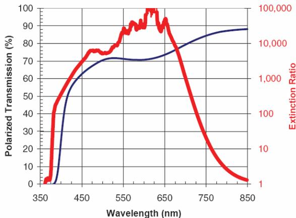
FIG. 1: A polarizer’s transmission and contrast ratio can be shown graphically against wavelength. The contrast ratio is determined by dividing the maximum transmission by the minimum transmission. By looking at the graph at different places, it can be seen that both specifications are wavelength dependant.
