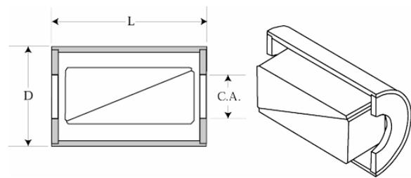
FIG. 5: A Glan-Thompson polarizer is an example of a crystalline polarizer.
