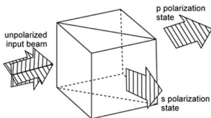
FIG. 4: A beamsplitting cube transmits the p polarization state through and reflects the s polarization state at 90 degrees.
