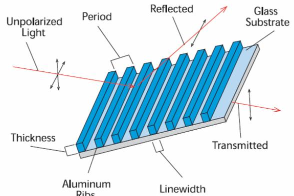
FIG. 3: A Wire Grid Polarizer transmits the P-polarized light and reflects the S-polarized light.
