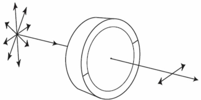
FIG. 2: A Dichroic polymer polarizer transmits only the desired polarization direction and absorbs the rest.
