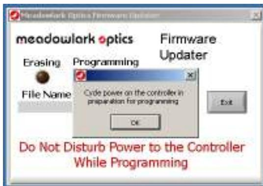
3. Cycle power on the controller to ensure the USB connection is properly made. Wait until the front panel status LED is done flashing before clicking OK. If the power is not cycled or the OK button is clicked before the front panel status LED is done flashing, the following error will be displayed. If this error appears, close the firmware updater program and re-run it.
