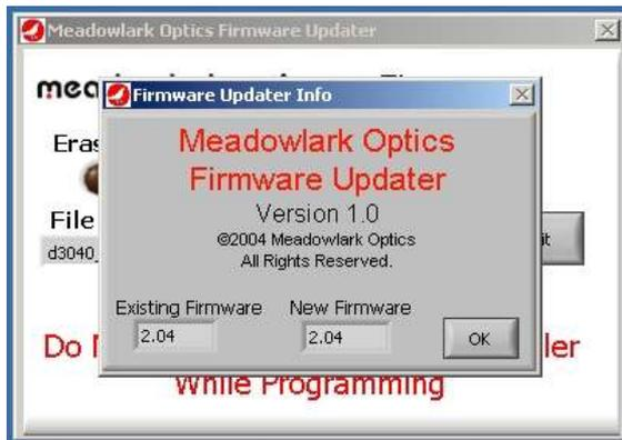
7. As the firmware is being erased and reprogrammed the status will be displayed as shown. **DO NOT disturb power to the controller while it is erasing or reprogramming.** If power is disturbed the controller's memory will be corrupted, requiring the unit to be returned to Meadowlark Optics for reprogramming.
