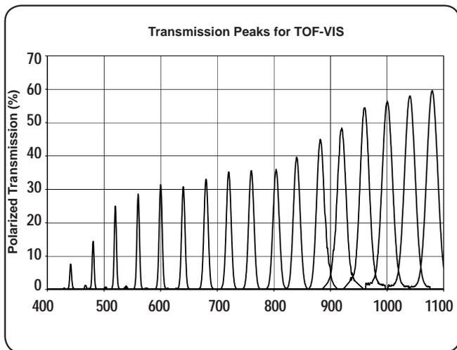
Fig. 7-2 Typical Filter curves for the TOF-VIS
