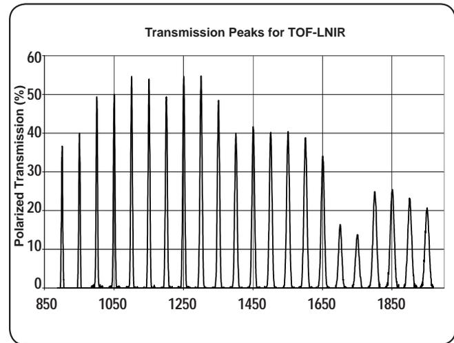
Fig. 7-3 Typical Filter curves for the TOF-LNIR
