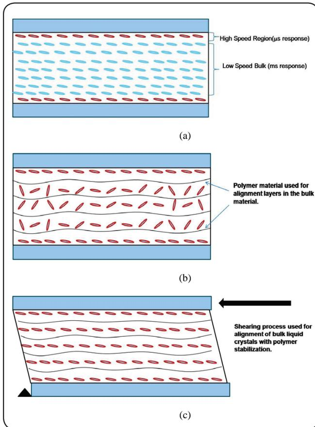
**Fig. 4-17** (a) Typical bulk liquid crystal device showing both regions of fast and slow electro-optical response.
