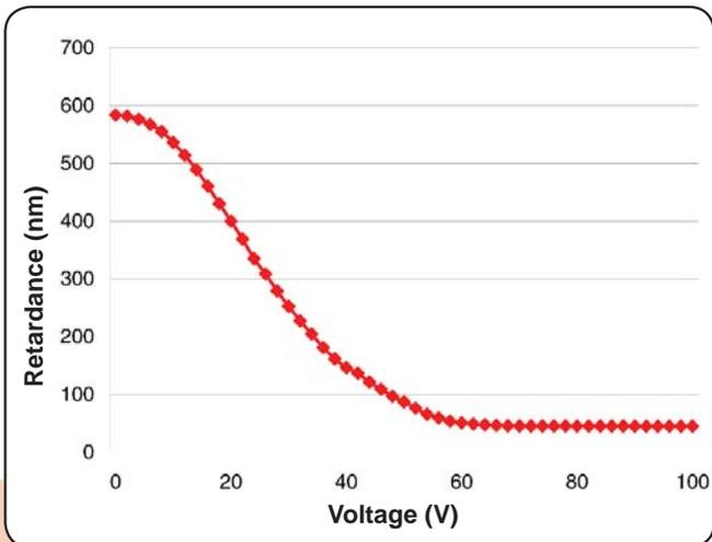
Fig. 4-19 Swift Liquid Crystal Retardance vs Voltage
