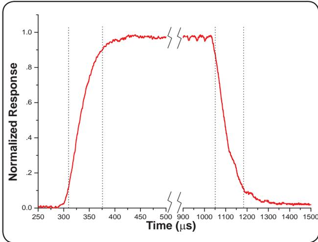
Fig. 4-18 Swift Liquid Crystal Response Time Plot
