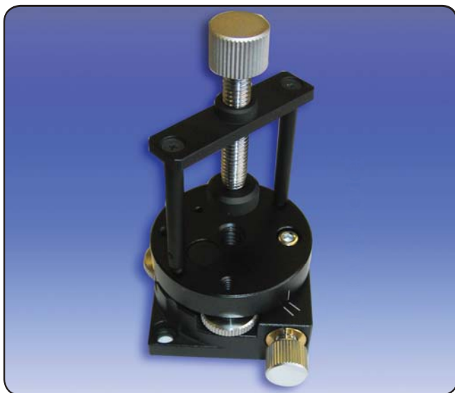
Fig. 3-3 32 mm mount 3-axis stage (tip, tilt and rotation)
