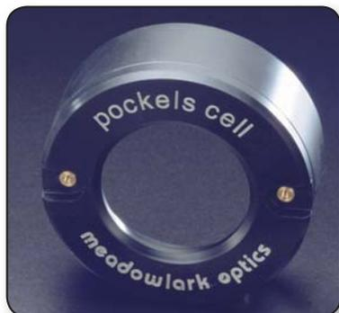
Our longitudinal Pockels Cells are often used in polarimetry on imaging light beams and in the chopping of polarized beams. They consist of Z-cut KD\*P crystals between protective windows that have transparent indium-tin oxide electrodes applied to their interior faces. The electrodes produce a
