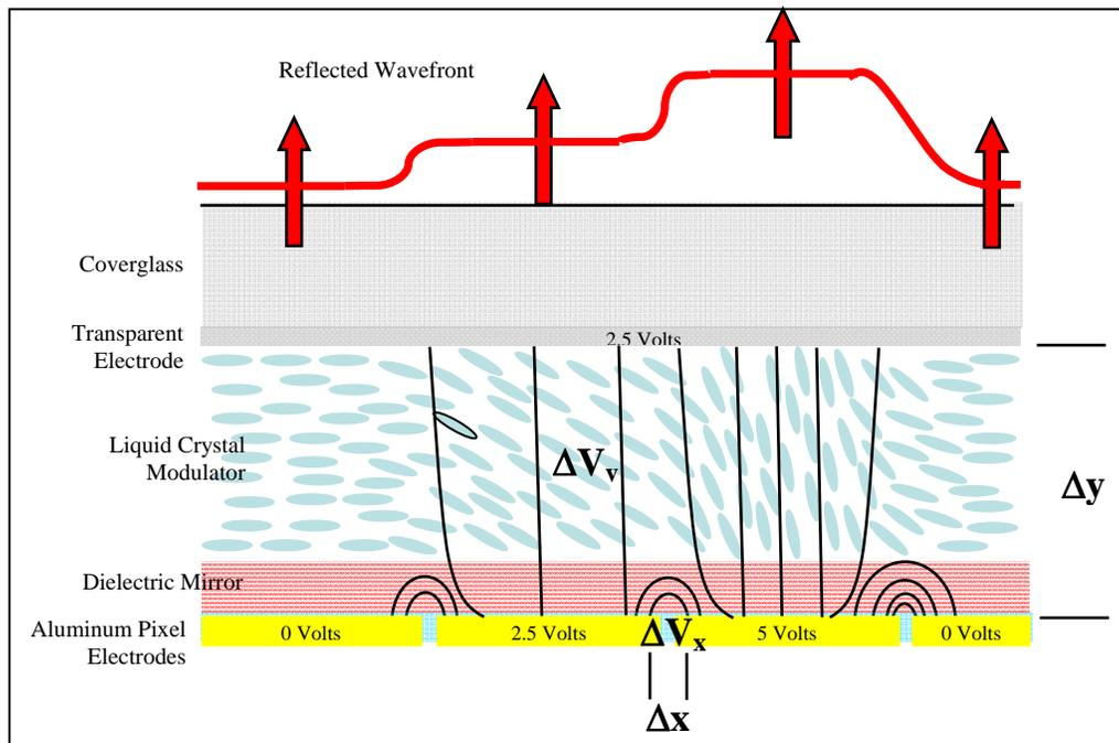
Figure 4 ~ Planarized dielectric mirror and smoothing of the electric field eliminate most of the grating effects associated with pixilated spatial light modulators.
