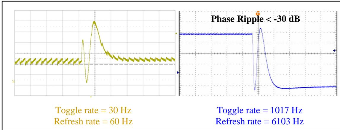
Figure 3 ~ ECB modulators addressed at different rates. The left trace shows a strong data-dependent ripple that is synchronous with the video rate addressing period. The right trace shows the ripple being suppressed by sub-millisecond refresh rates.
