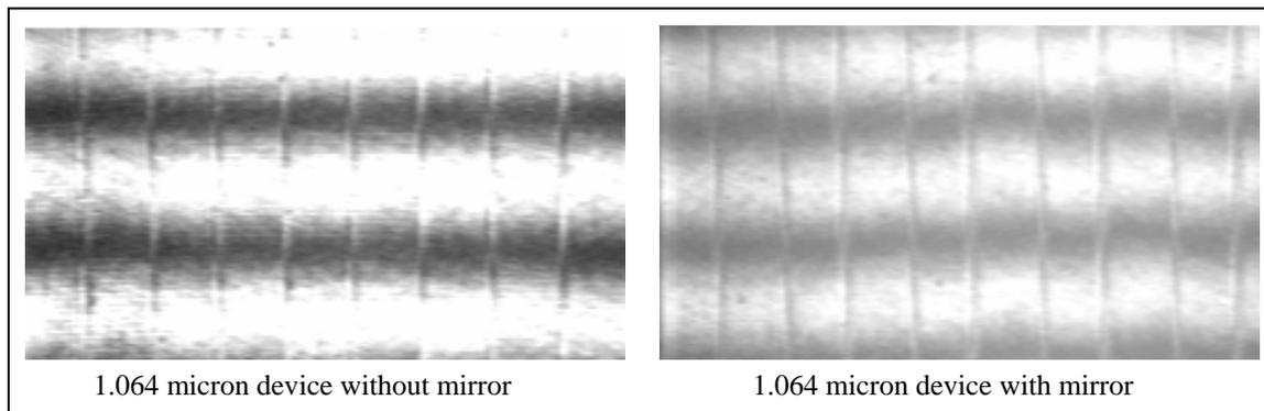
Figure 2 ~ Interferometer images of two 512 x 512 SLMs (left – without mirror, right - with mirror) operating at 1064 nm. The pattern written to the SLM has 15 pixels set to zero phase and 16 pixels set to  $2\pi$  phase. The discontinuities in the horizontal fringe pattern show the relative width of the  $2\pi$  transitions.
