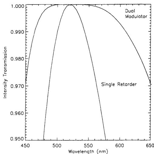
Fig. 2. Theoretical comparison of the bandwidth of the on state of the dual SmA\* modulator with the transmission of a single SmA\* half-wave retarder between crossed polarizers and oriented at  $45^\circ$  with respect to the incident polarization.
