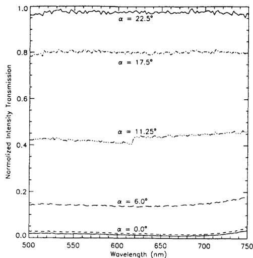
Fig. 4. Experimental transmission spectrum for the reflection-mode analog intensity modulator with a single SmA\* device and a compound achromatic quarter-wave retarder. Normalized intensity measurements are parameterized by the difference angle  $\alpha$ .
