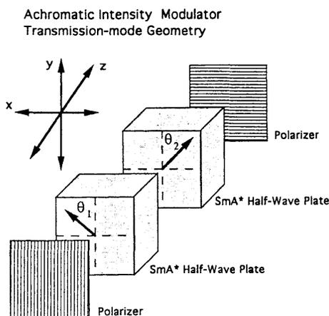
Fig. 1. Schematic for a broadband analog intensity modulator based on a dual SmA\* polarization rotator. The angles  $\theta_1$  and  $\theta_2$  are the absolute orientations of the retarder optic axes with respect to the incident  $\hat{y}$ -polarized light.
