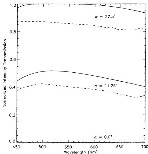
Fig. 3. Comparison of theoretical (solid curves) and experimental (dashed curves) transmission spectra for the analog intensity modulator parameterized by the difference angle  $\alpha$ .
