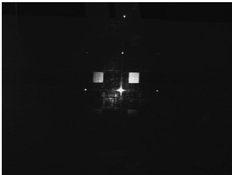
**Figure 9.** Diffraction pattern from an SLM with a dielectric mirror on its backplane addressed to produce a 9x9 array of spots in the +1, +1 order.
