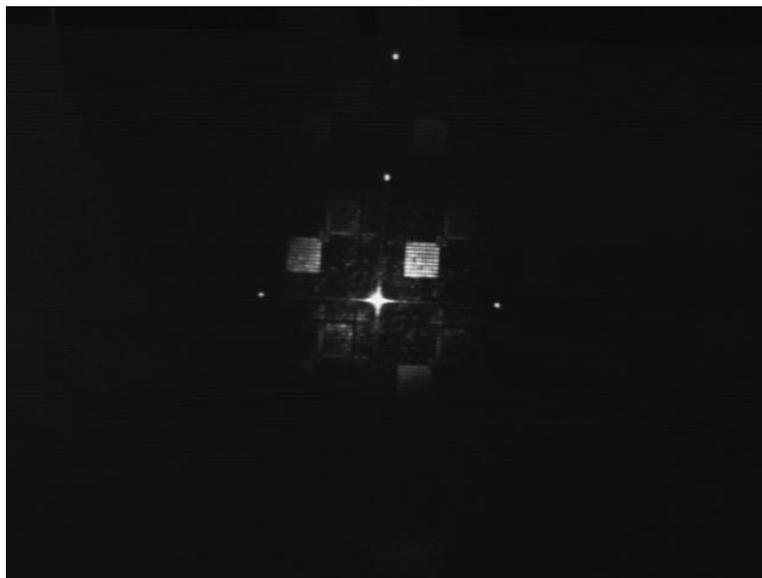
**Figure 8.** Diffraction pattern from a non-mirrored SLM addressed to produce a 9x9 array of spots in the +1, +1 order.
