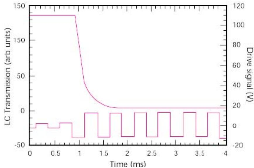
Figure 2: Half-wave relaxation time (a) and rise time (b) for the cell of Fig. 1.
