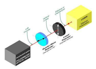
Figure 1 – Schematic for Polarimeter Calibration, Step 6
