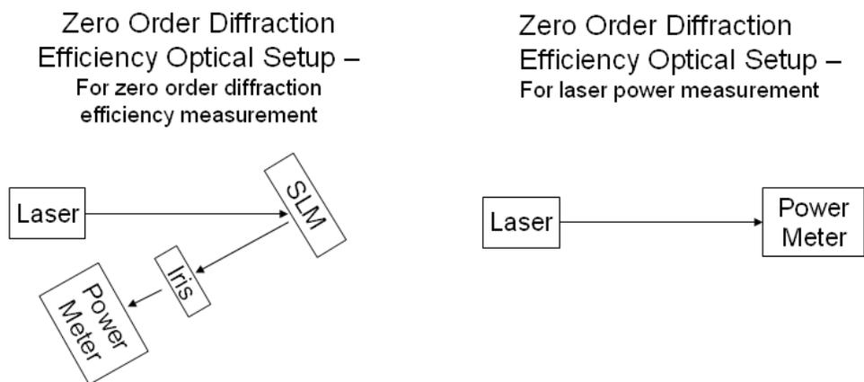
Figure 5 – Optical layout used to measure 0<sup>th</sup> order diffraction efficiency.
