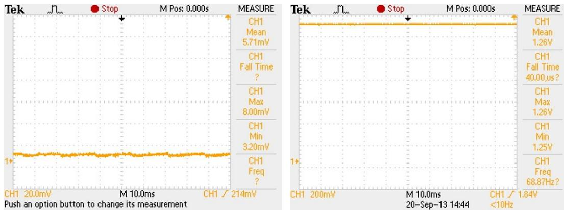
Figure 3 – (left) Solid pattern resulting in an off state = 5.71 mV (right) solid pattern resulting in an on state = 1.26 V
