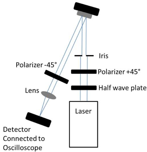
Figure 1 – Slightly off axis configuration to use the Nematic SLM as an amplitude modulator.
