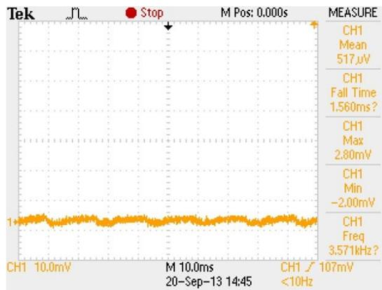
Figure 4 – background noise with laser blocked = 517  $\mu\text{V}$
