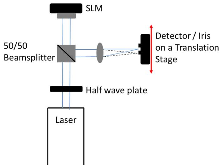
Figure 6 – Optical layout used to measure 1<sup>st</sup> order beamsteering efficiency.
