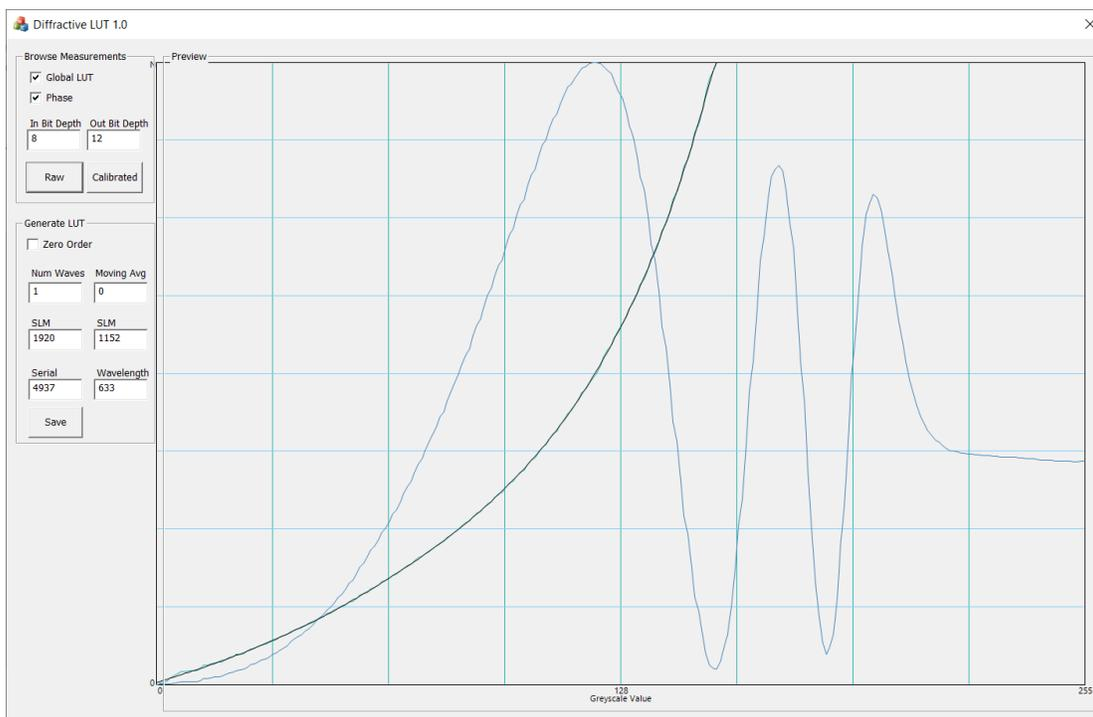
Figure 7 – Intensity measurements are recorded as diffraction gratings are loaded to the SLM. By post processing the intensity measurements the modulation depth of the SLM can be determined.
