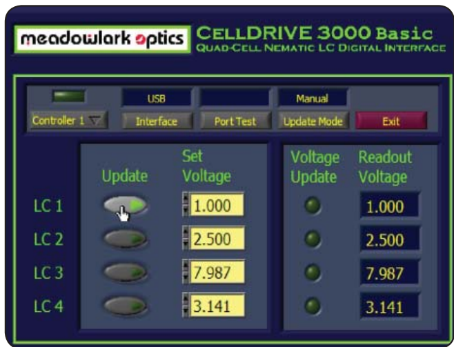
Fig. 5-2 Basic D3040 operation enables computer control for up to four Liquid Crystal Variable Retarders
